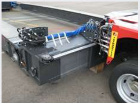
Widenable boiler deck
