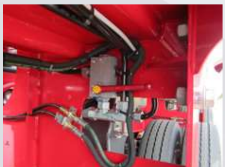
Hose rupture safety valve
