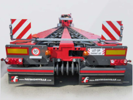
Lighting with underrun
