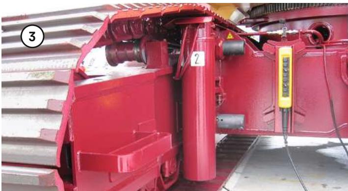
1 Transport without crawlers Transport sans longeron
