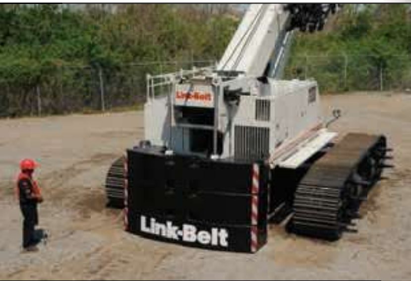
Fast, easy counterweight removal
