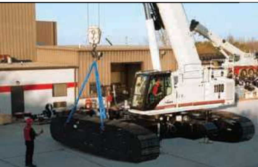
Fast, easy counterweight removal
