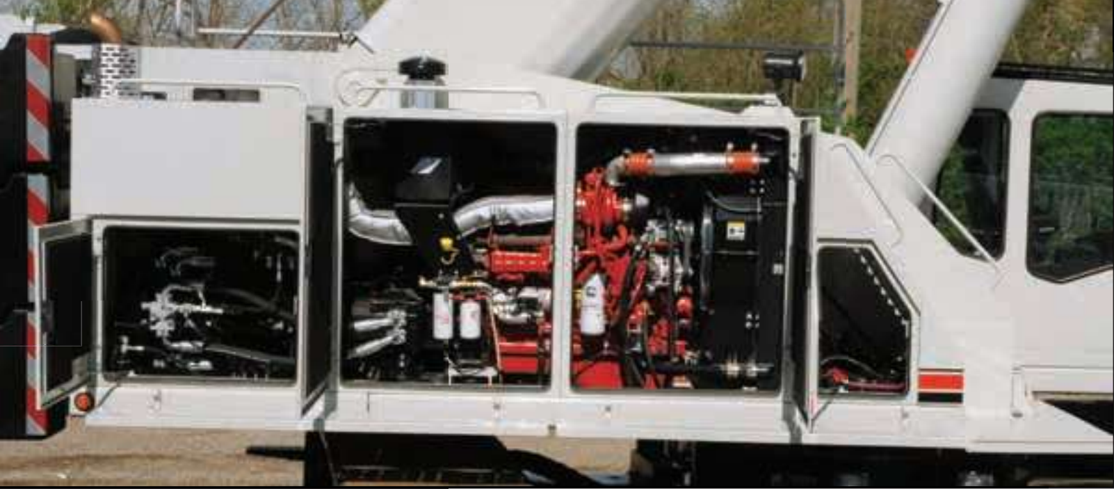
Excellent access for all routine engine and hydraulic maintenance
