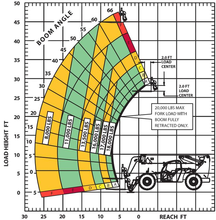
LOAD RATINGS ARE FOR VEHICLE EQUIPPED WITH FOAM FILLED OR SOLID TIRES.
